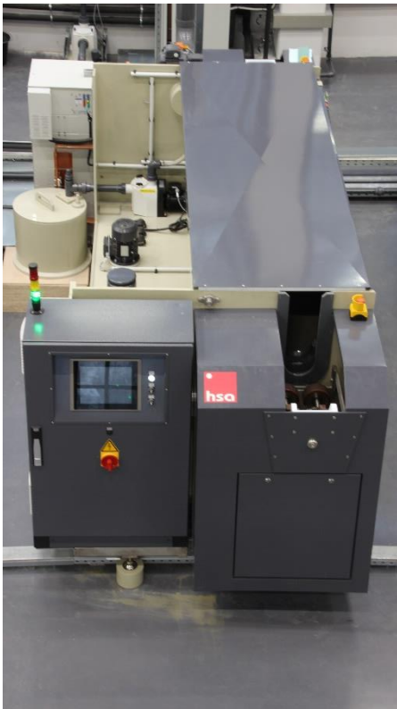
Degreasing tank: degrease, decap if necessary, applying separation solution
