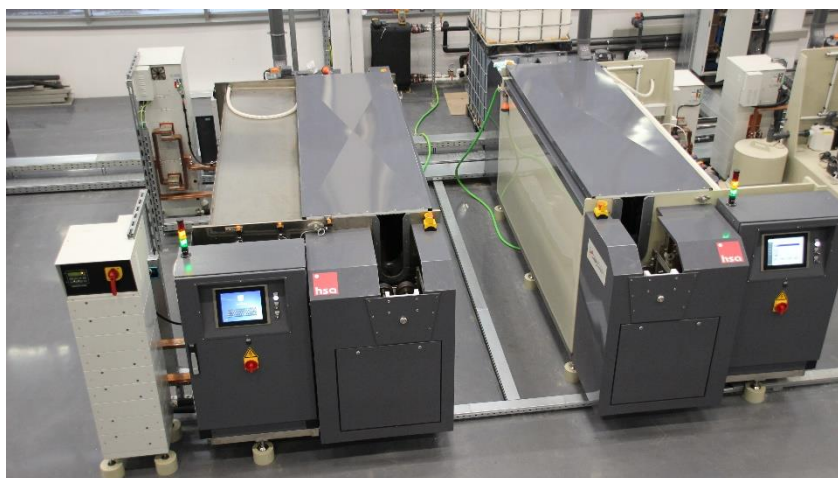
Chrome tank (left, with 2 rectifiers) and Copper tank
