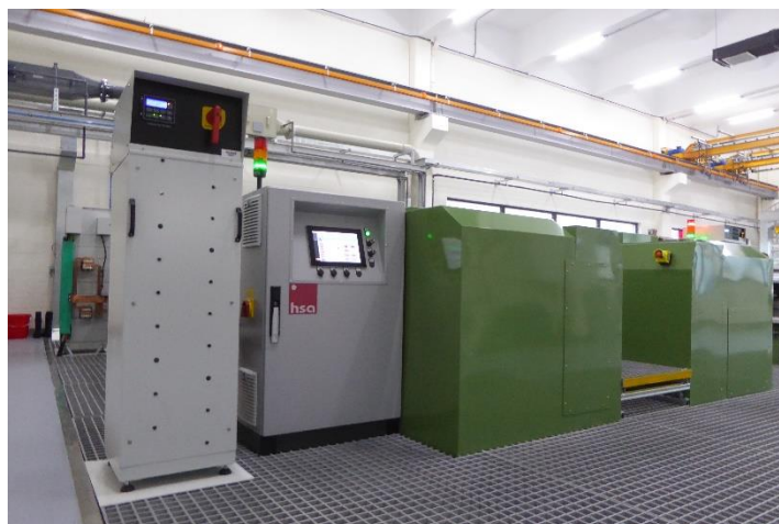
Chrome tank (left side with 2 rectifiers) and Dechrome tank
